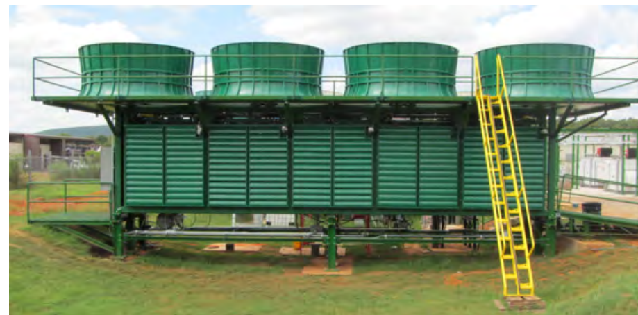
→ Global Thermostat direct air capture pilot unit.
